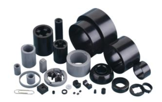
Bonded neodymium magnets are usually compact isotropic magnets, they can be magnetized multi-polar and made into complex shapes which are difficult to be realize on sintered neodymium magnets and have tight tolerances, no need for further mechanical machining.
